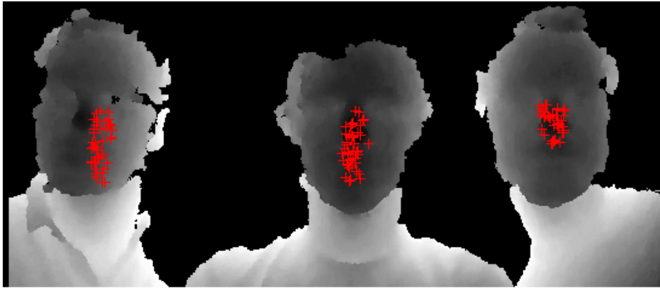
Figure 4.4: Structure candidates found during random sampling (Depth Image). The image is a 16-bit image, and the depth values have been scaled to maximize the dynamic range of 0-65535.
