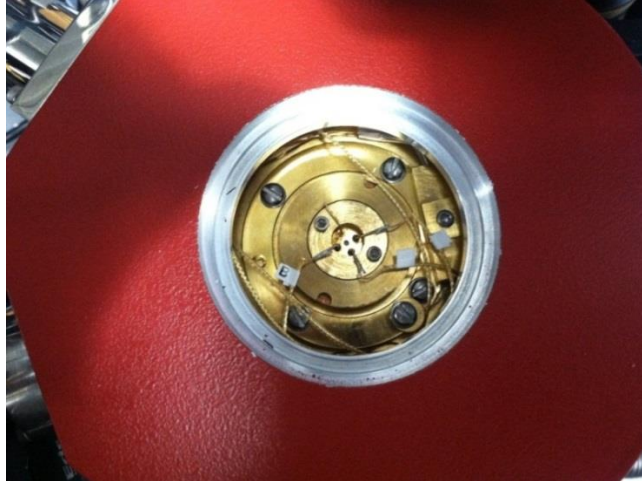
Figure 24: A picture of the HEMT device mounted inside the cryostat and oriented so that IR-radiation was passing through the grating first.
