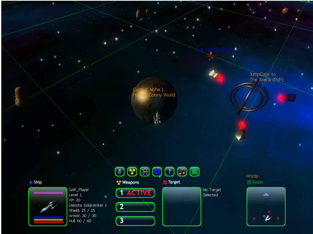
Figure 6.15: GAR Spatial Hashing. The spatial hashing methods in GAR are based on two papers I co-authored [MG05, HMG04]. To optimize rendering, collision, picking, sound effects, particle special effects, and AI routines in GAR, each system in GAR is divided into grid cells called sectors (shown above). Every frame, all objects in the game are placed into grid cells by a hash function. This spatial hashing routine optimizes nearly all aspects of the GAR game engine, including rendering, collision, NPC decision routines, picking, sound effects, and special visual effects.
