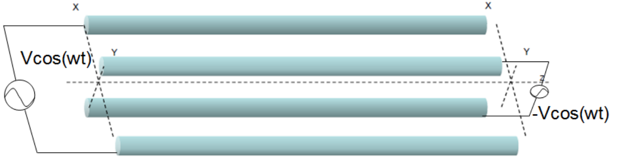
Figure 27: Linear quadrupole ion trap
