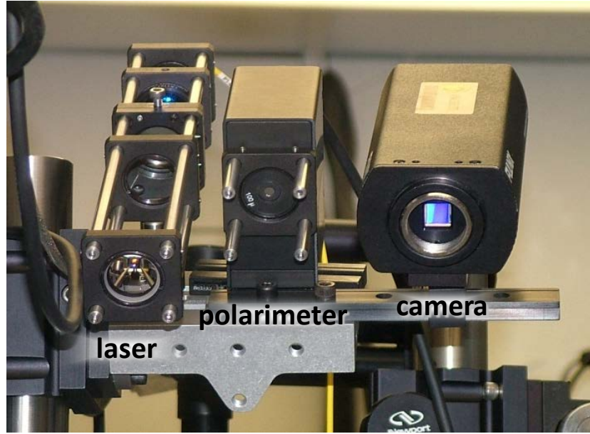
Figure 3.1: Illumination and detection set-up for measuring scattering from asphalt samples.
