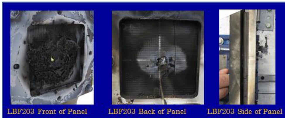
Figure 30. Panel LBF203 Post Test
