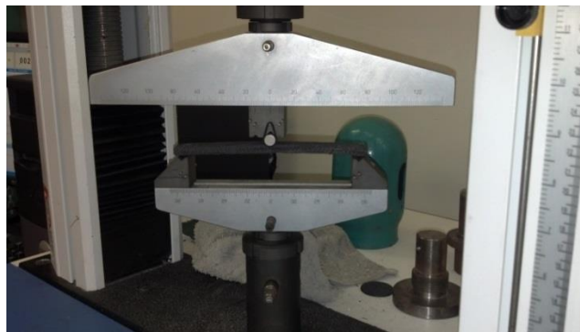
Figure 25. 3 Point Bend Test Setup
