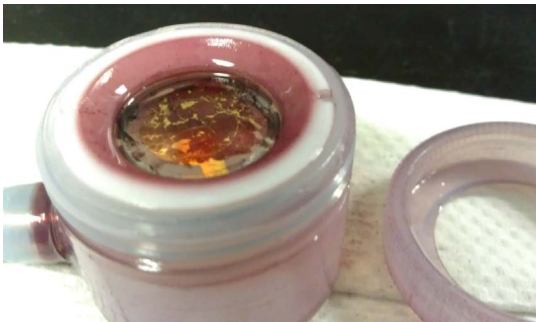
Figure 10. Image of the P3HT grown onto graphene deposited onto the QCM stage. Note the cracks in the graphene during transfer are clearly evident, as P3HT has deposited quite selectively onto the graphene portion.
