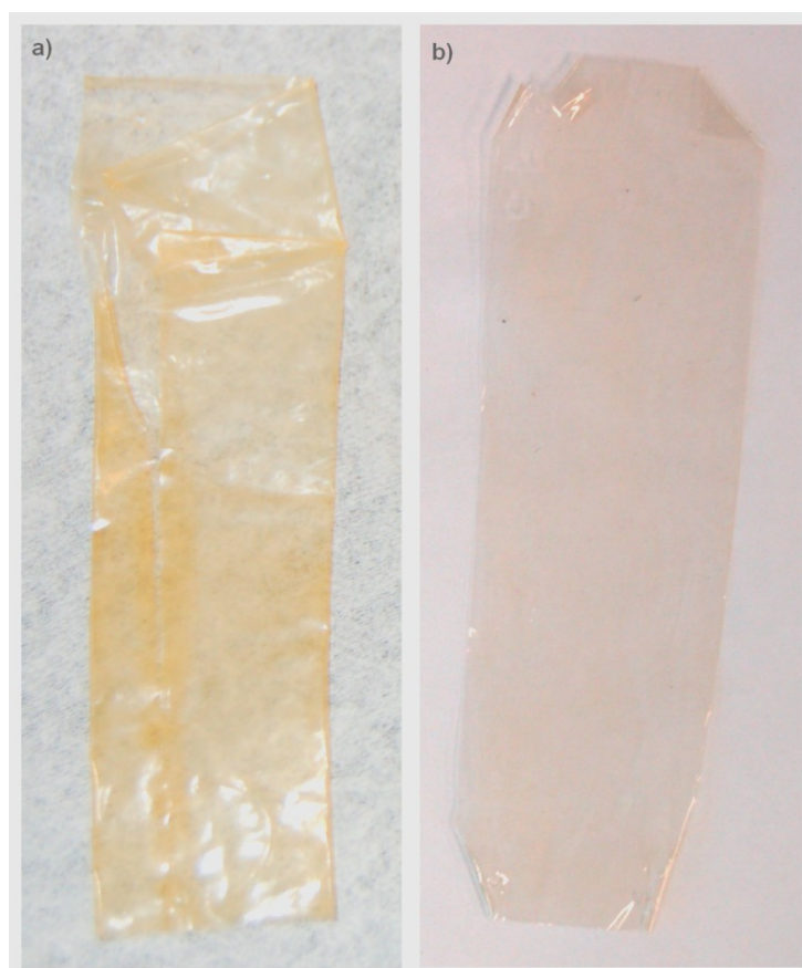
Figure 37 GF tested membrane after drying in oven: a) baseline and b) synthesized 2.0 wt%
