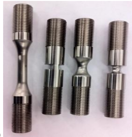
(a) (b) Figure 17: (a) Symbol notation of the cross section of a notched specimen (b) Four different shapes of the specimens before fracture.
