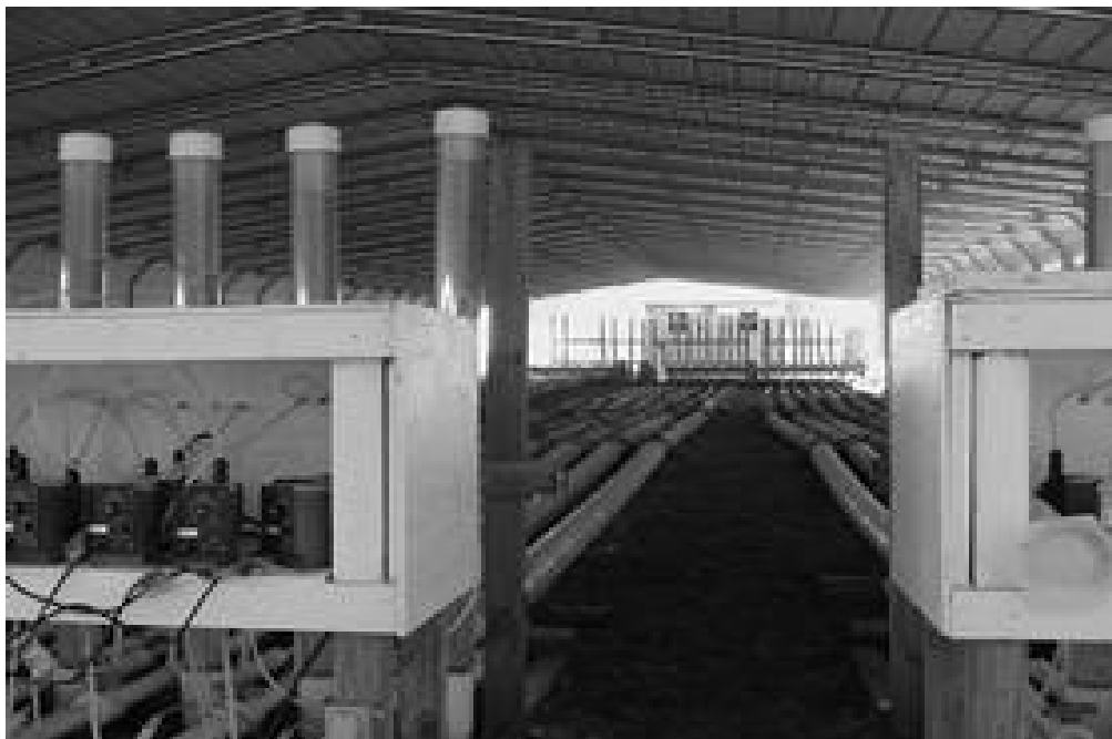
Figure 3.2 Pilot Distribution System Headwork
