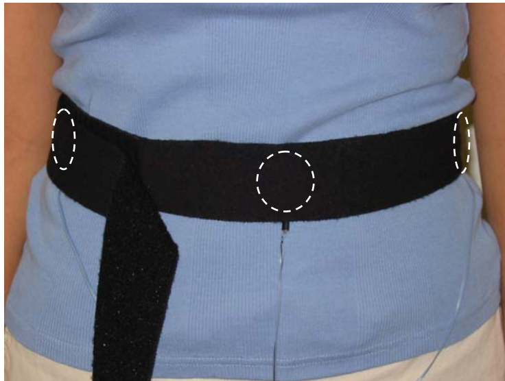
Figure 7. The three-tactor array, as worn by a participant. The dotted-lines show the approximate locations of the tactors.
