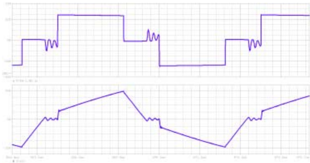
Fig. 5.17 (c) With active-clamp snubber ( C_s=3\mu\text{F} )
