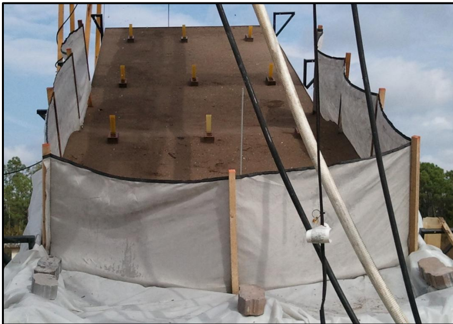
Figure 2 Nonwoven (BRSF) silt fence fabric installed on a tilted test bed
