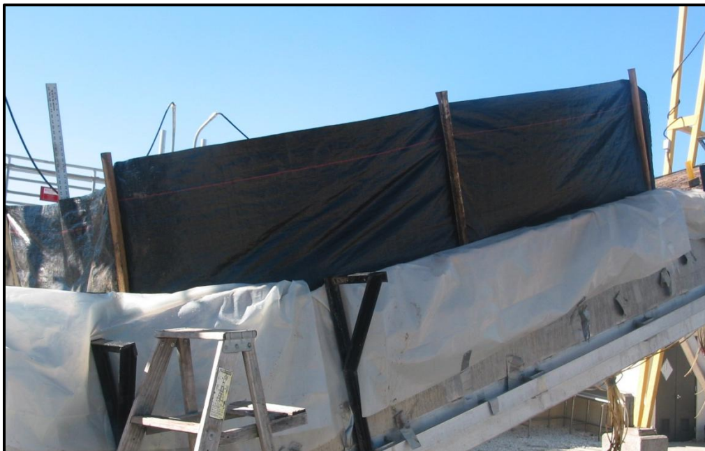
Figure 1 Woven silt fence fabric installed on a tilted test bed
