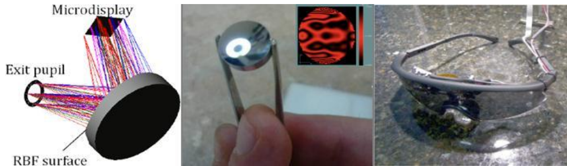
Figure 12 RBF optical surfaces in compact HWD design [32, 33].
