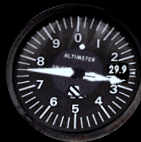
A pointer with a needle tip showing 100 foot intervals
