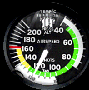
The ASI indicates a speed of 120 knots
