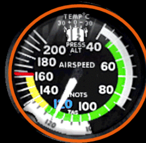
The ASI indicates a speed of 120 knots
