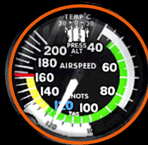
The ASI indicates a speed of 120 knots
