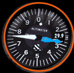
A pointer with a flared triangular tip showing 1,000 foot intervals
