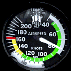
The ASI indicates a speed of 80 knots
