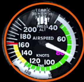
The ASI indicates a speed of 80 knots
