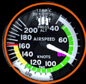
The ASI indicates a speed of 80 knots
