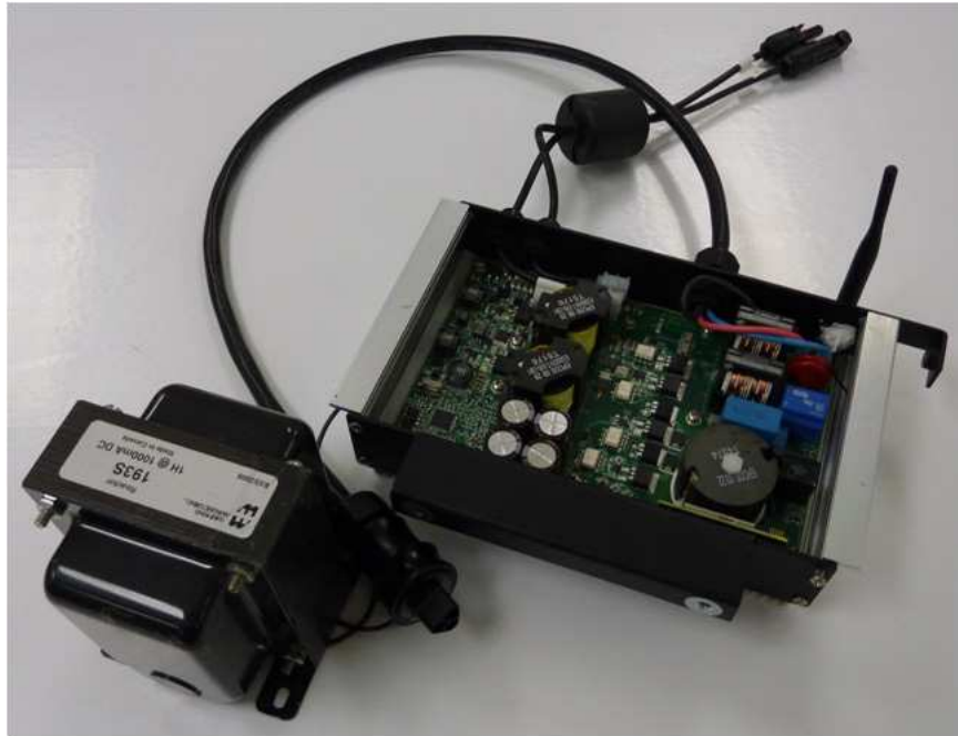
Figure 1.9: Comparing the size of a large inductor and an actual micro inverter, courtesy of Petra Solar Inc.
