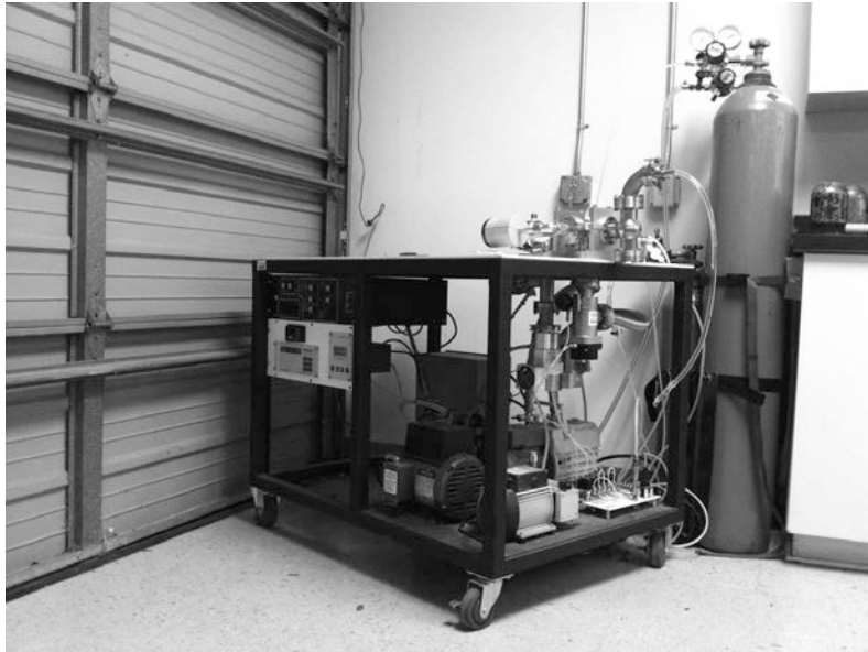
Figure 5. High vacuum system for evacuating quartz capsules.
