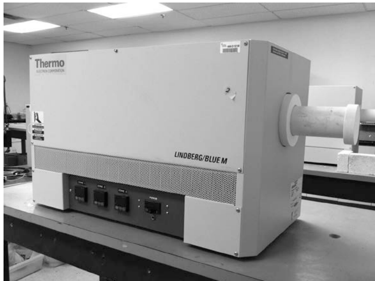
Figure 6. Lindberg/Blue™ three-zone tube furnace
