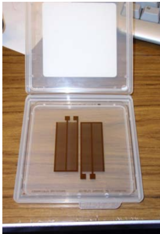
Figure 26. Mask for the fabrication of DEP electrode wafers
