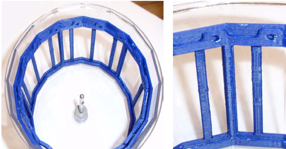
Figure 28. Rapid Prototype for slotted wafer holder
