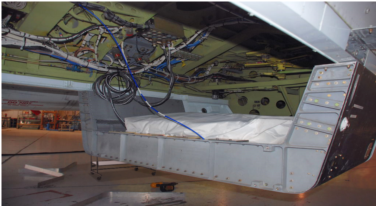
Figure 2.4 HIRAD in the flight pallet.
