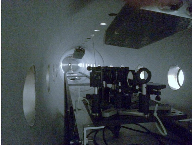
Figure 2.6: Grazing incidence filament beam profiler on the rail inside CLaPTAM
