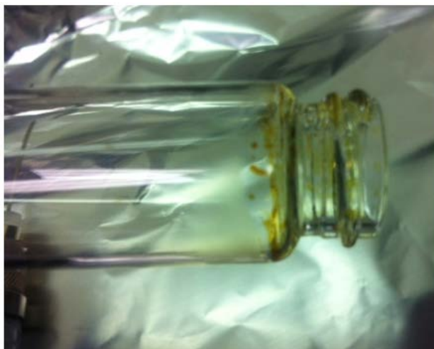
Figure 29: Pyrex vial with vapors condensed at the front end
