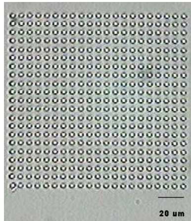
Figure 3.10: Optical microscope image of voids created in the volume of borosilicate glass through femtosecond laser direct writing.
