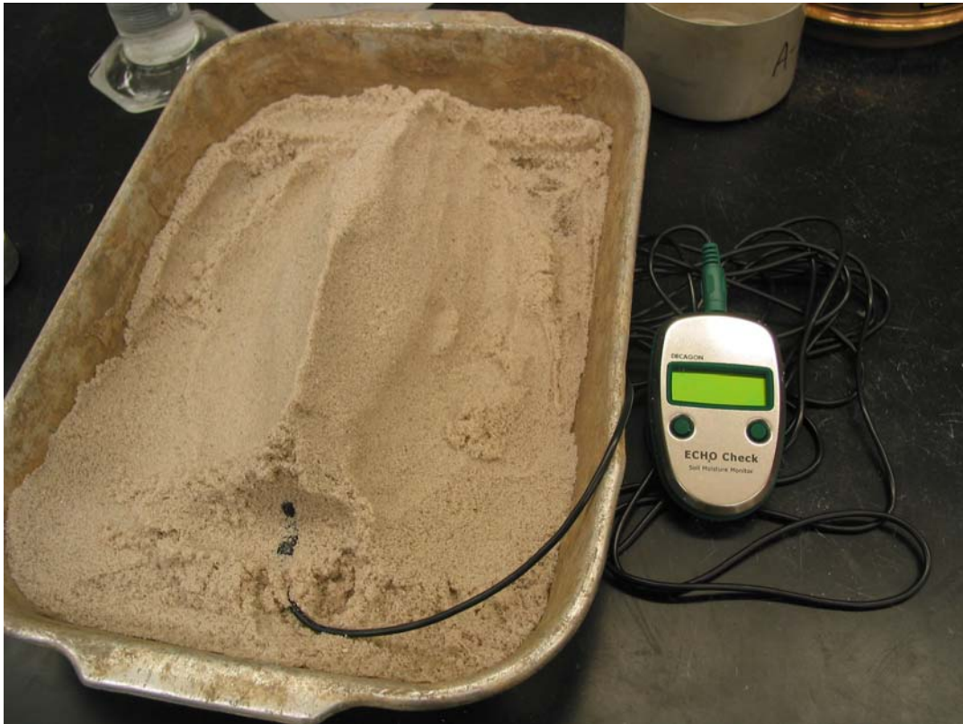
Figure 6: ECH2O Probe Calibration in Progress
