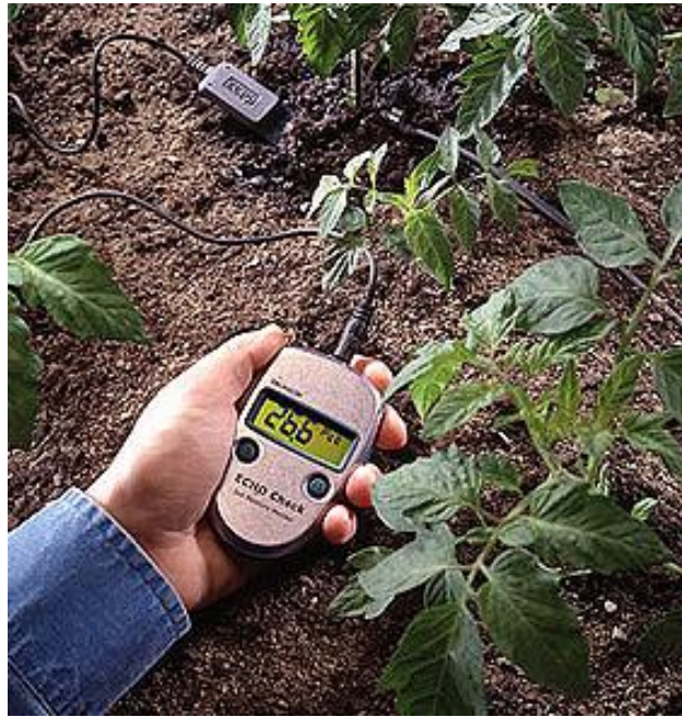
Figure 2: ECH2O Check Display Device
