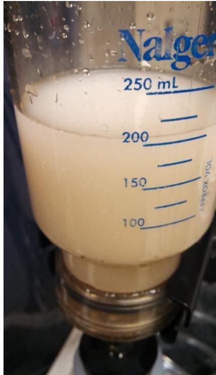
Figure 57. Photograph of the Filtration of RCA Fines from Water
