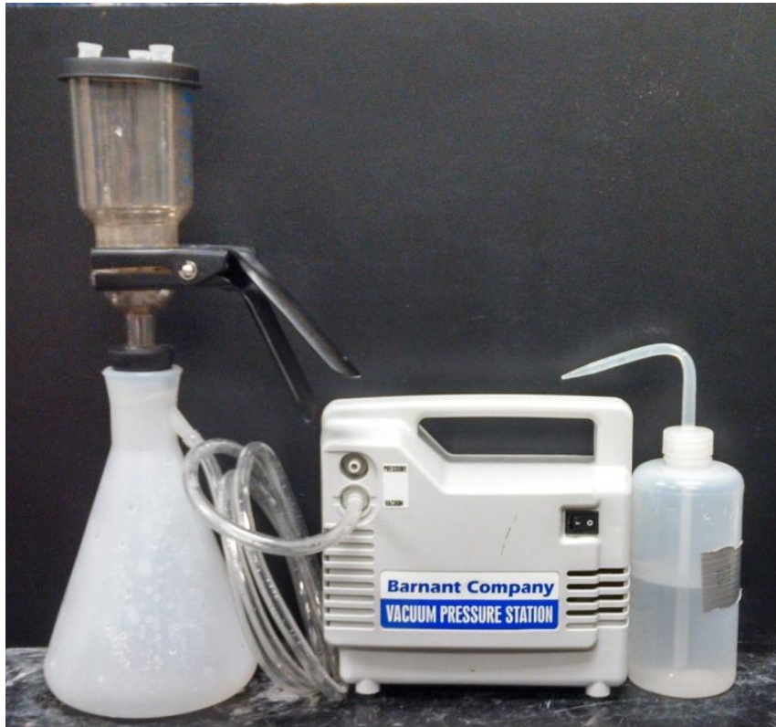
Figure 55. Filtration Equipment Required for ASTM D5907
