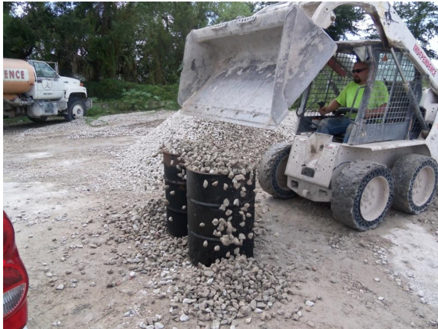
Figure 7. RCA Being Obtained from an Orlando, FL Recycling Facility
