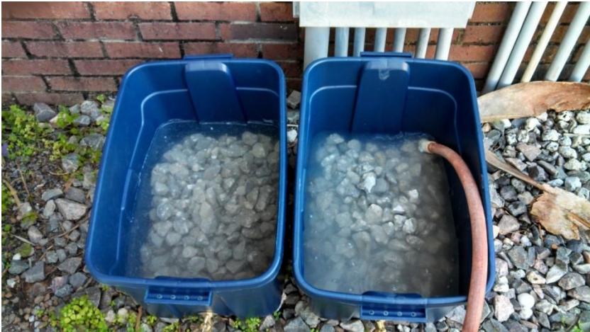
Figure 15. Aggregate Washing Setup
