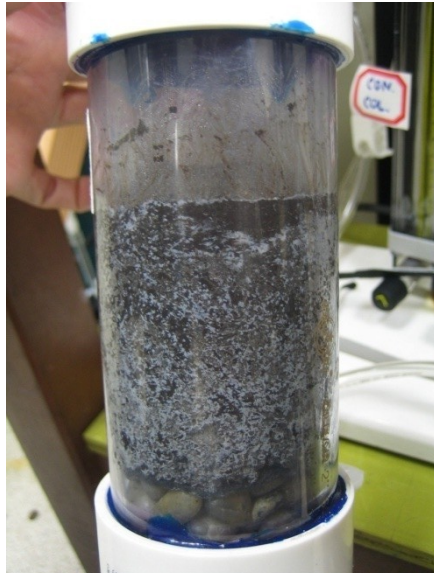
Figure 3-4. White powder appeared in the autotrophic nitrification column at high H 2 S loading.
