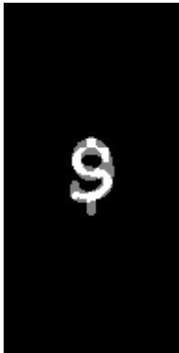
Figure 34: Difference of aligned characters; in white shown overlapped parts and in grey shown parts that did not overlap
