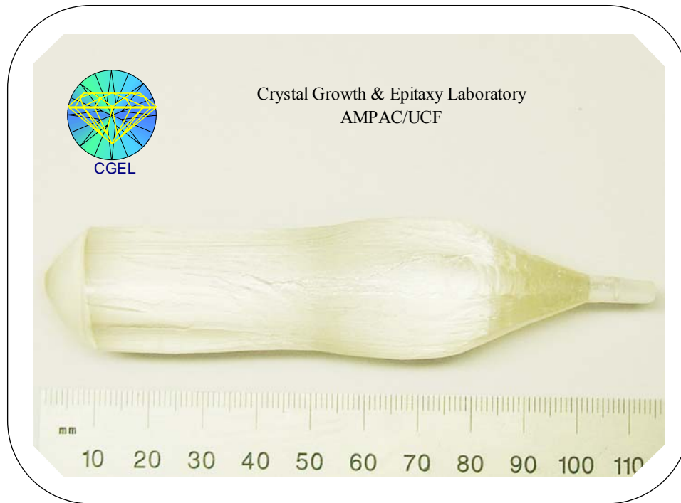
Figure 6-15: Crystal-10 growth by LRPC-MPC
