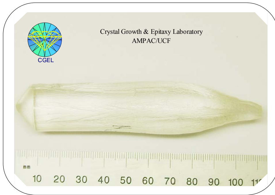
Figure 6-18: Crystal-11 growth by LRPC-MPC
