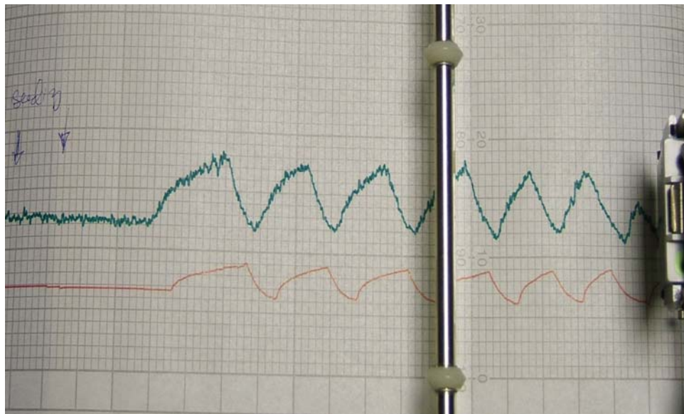
Figure 5-8: Cooling water and chilled water temperature fluctuations
