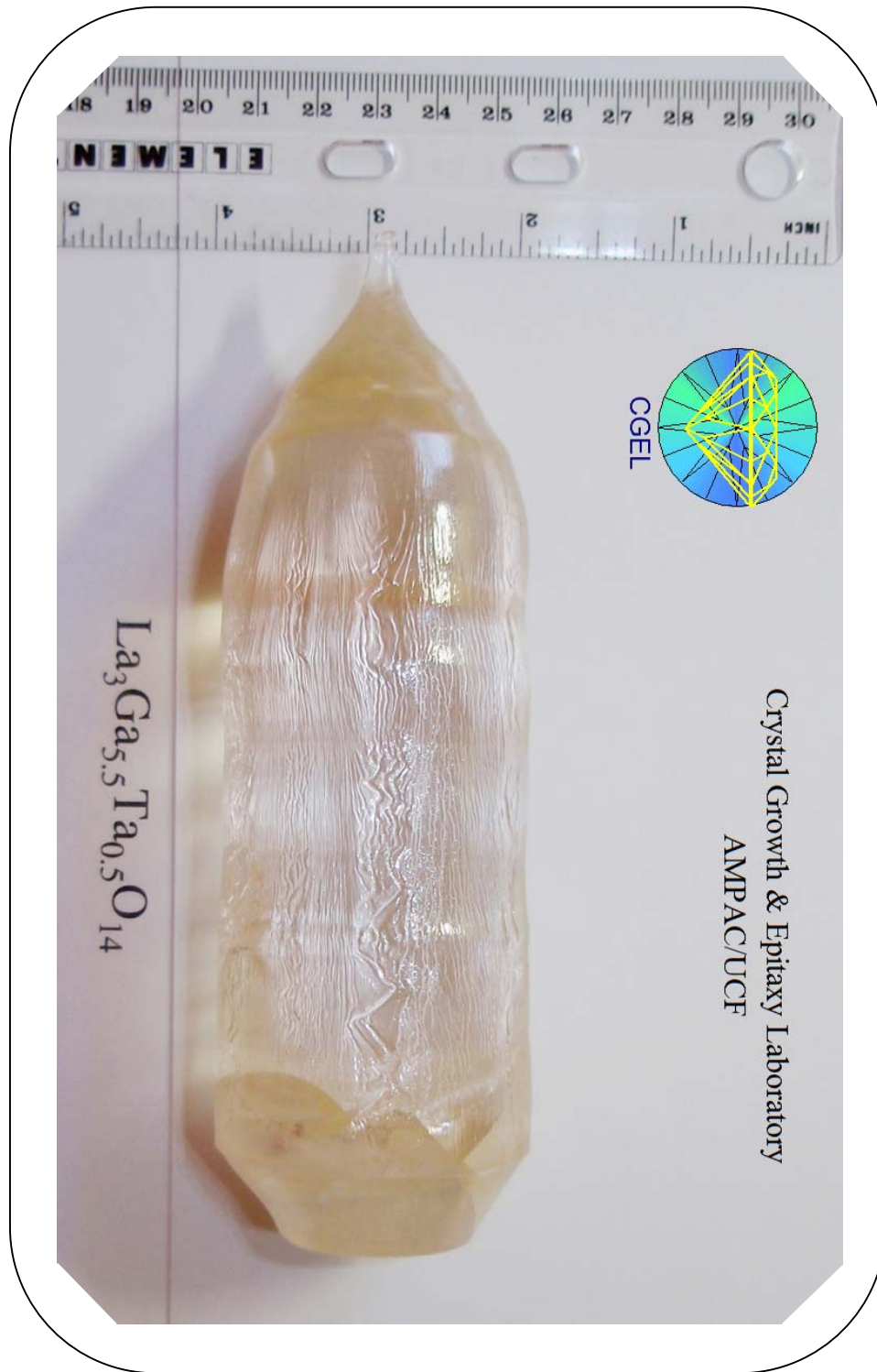
Figure 6-21: Crystal-12 growth by LRPC-MPC
