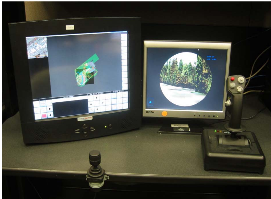
Figure 9. Simulated Gunnery and Tactical Control Unit. The TCU and gunnery station is located on the left and right, respectively.
