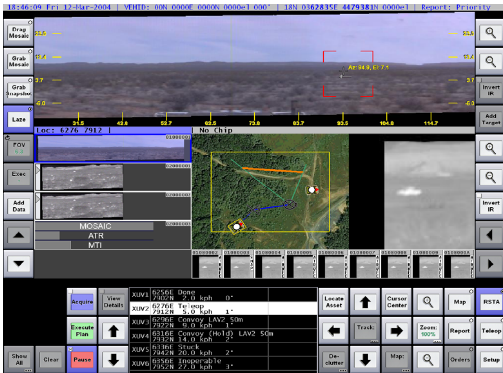
Figure 8. User interface for Robotic Tactical Control Unit TCU
