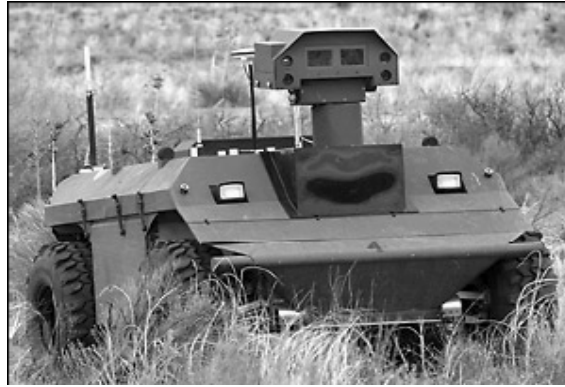
Figure 5. The Experimental Unmanned Ground Vehicle (XUV) (Schipani, 2003).
