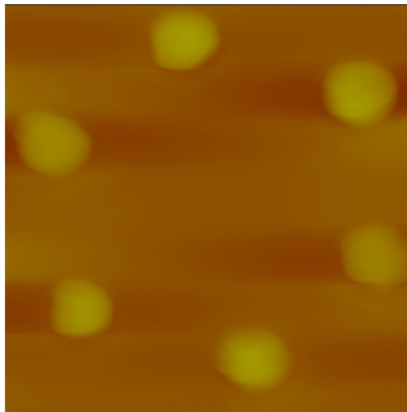
Figure 3-12 AFM image of gold nanoparticles after polystyrene nanospheres removed and annealed at 600°C for 1 hour.
