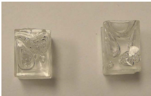
Figure 4-2: Fully polymerized PMMA samples. No crystal particles were included in this sample. Many bubbles can be seen trapped inside the samples.
