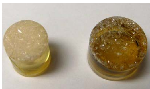
Figure 4-7: Fully polymerized PFCB samples (curing temperature \sim 220 °C). Many cracks were generated between particles and polymer. The sample on the right includes fewer particles than to the sample on the left.
