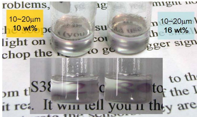
Figure 4-20: 2%Er:KY 3 F 10 powder in the index matched Polymer-gel. Different weight percents of crystal particles were suspended in the polymer and transparency was retained.
