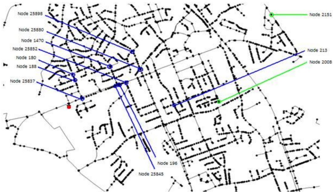
Figure 3.1. Section 2 of the network. Green and blue circles represent the nodes selected for chlorine residual and lead scenarios, respectively. The red dot represents Tank 26653 in which lead is injected to simulate the third scenario. The nodes selected for chlorine residual and lead scenarios, are represented in green and blue circles respectively.
