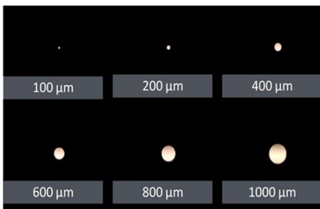
Images of Capillary Tube Recorded at Various Pinhole Diameters
