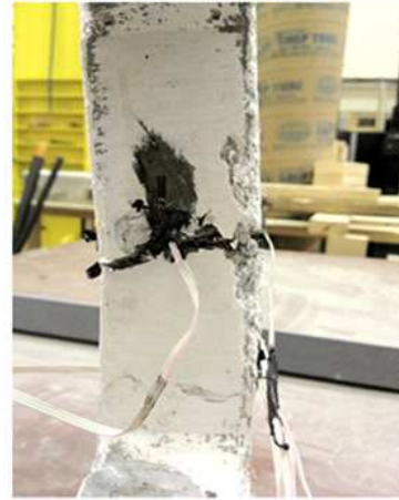
Strain Gage failure Closeview
