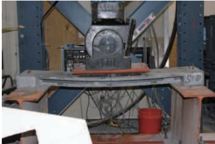
Figure 4.9: “UHPC-MMFX” specimen prior to failure
