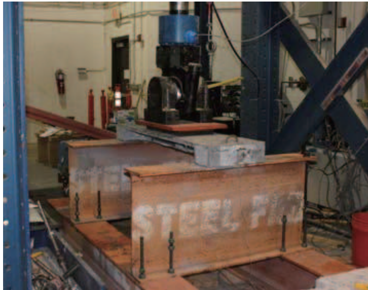
Figure 4.7: Test setup and instrumentation of “UHPC-MMFX” specimen
