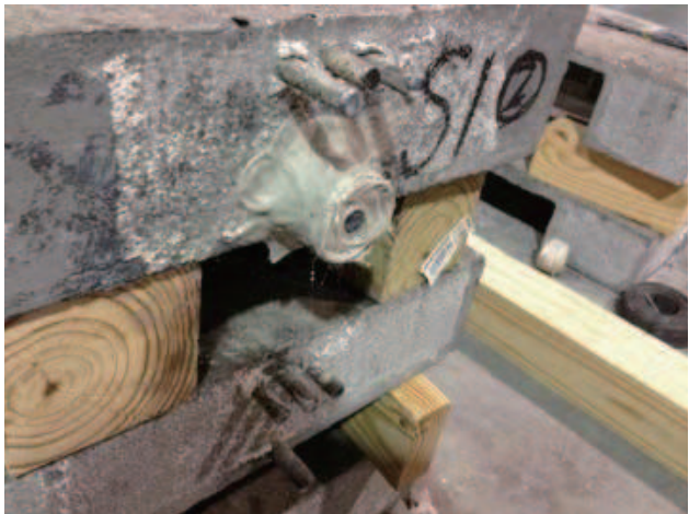
(a) End anchorage for CFRP Rods
