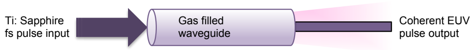
Figure 2.5: Femtosecond laser is focused into a gas filled waveguide to produce coherent EUV output
