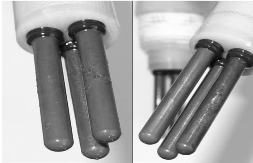
Photograph 4.3 Copper electrodes, left OP (1 mg P/L) and right ZOP (2 mg P/L).
