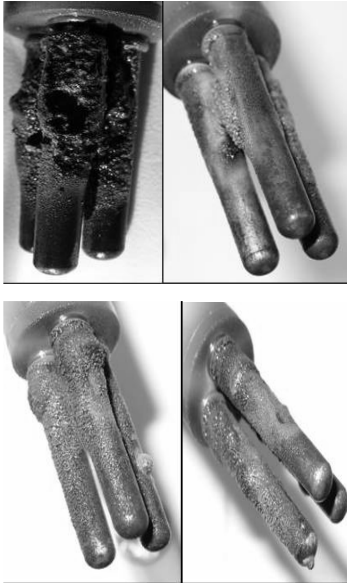
Photograph 6.3 Fe electrodes, clockwise from top left BOP ( 0.5 mg P/L), ZOP (2 mg P/L), \text{pH}_{\text{s}} and \text{pH}_{\text{s}+0.3} .
