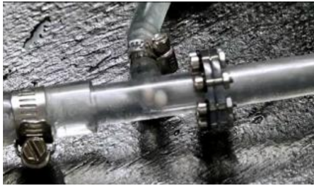
Figure 18: Rapid prototyped injection system introducing particles to flow loop.
