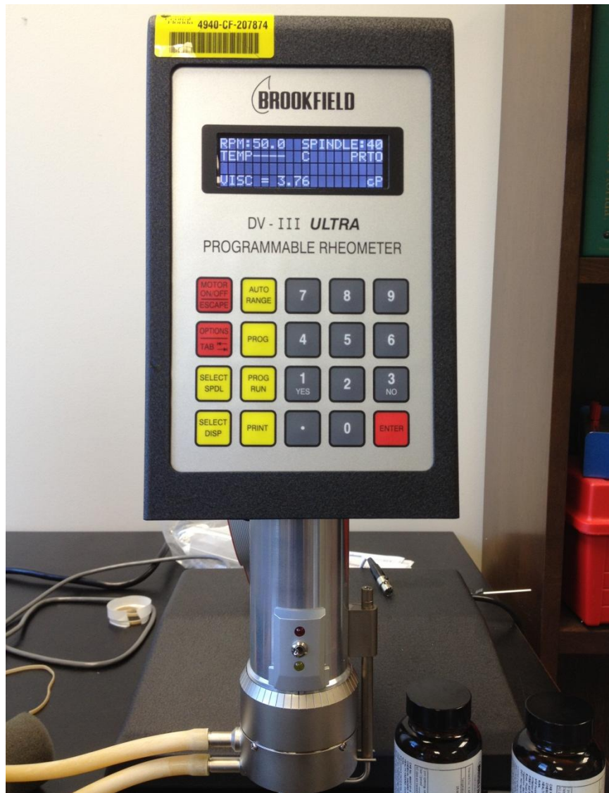
Figure 12: Viscometer with verified viscosity measurement.
