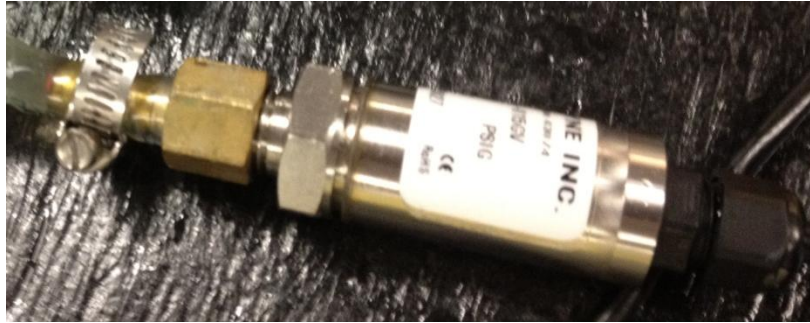
Figure 16: Pressure transducer attached near descending aorta.
