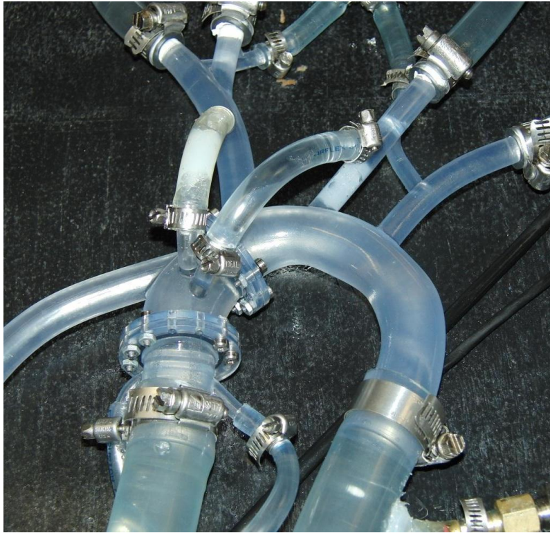
Figure 33: Shallow with LCA bypass and occluded LCA.
