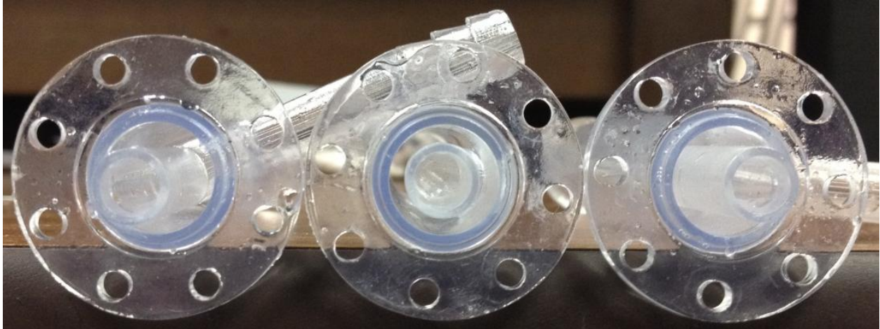
Figure 20: Three injection entry configurations, from left to right: inside, centered, and outside.
