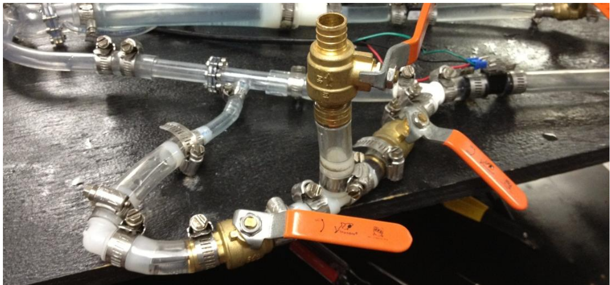
Figure 19: 3-valve injection system.
