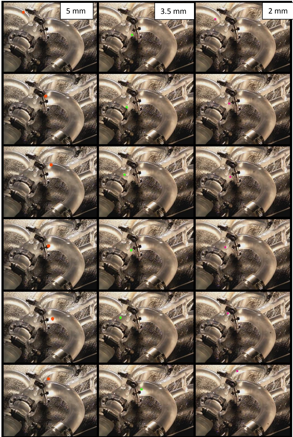
Figure 34: Particle tracks for perpendicular with LCA bypass.
