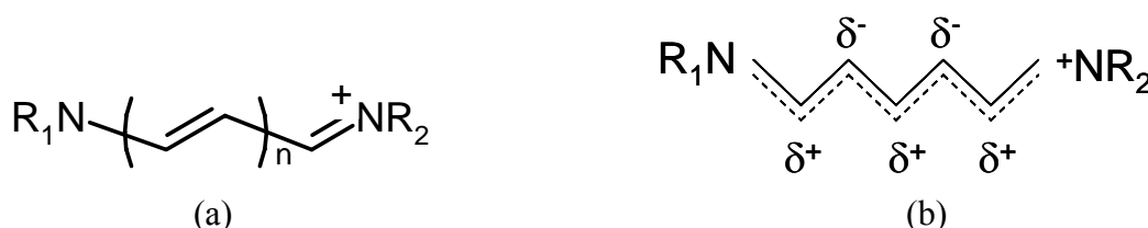
Figure 4.1 (a) General molecular structure of PD, R_1 and R_2 are terminal groups; (b) \pi -electron distribution in polymethine chromophore.
