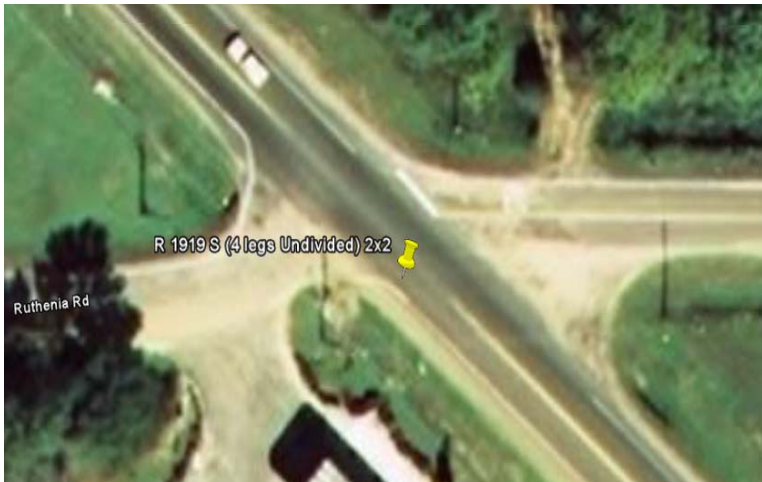
Figure 3-10: A 2x2 Four-Legged Unsignalized Intersection with an Undivided Median
