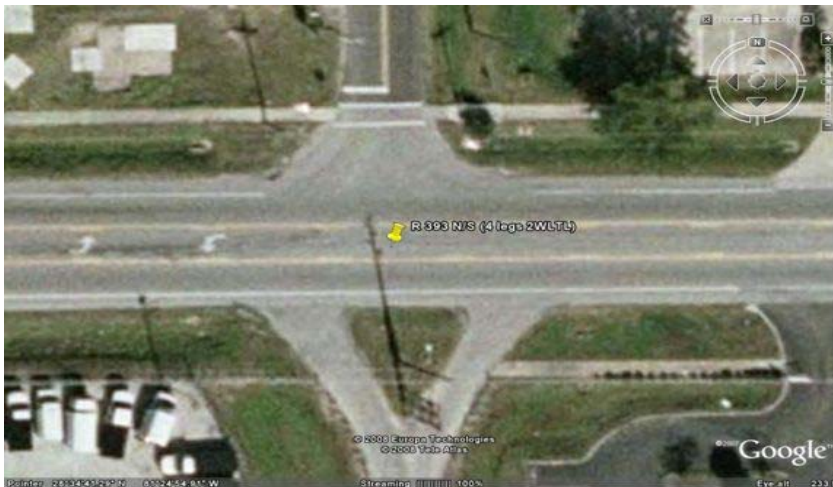
Figure 3-8: A 2x2 Four-Legged Unsignalized Intersection with a Two-Way Left Turn Lane Median
