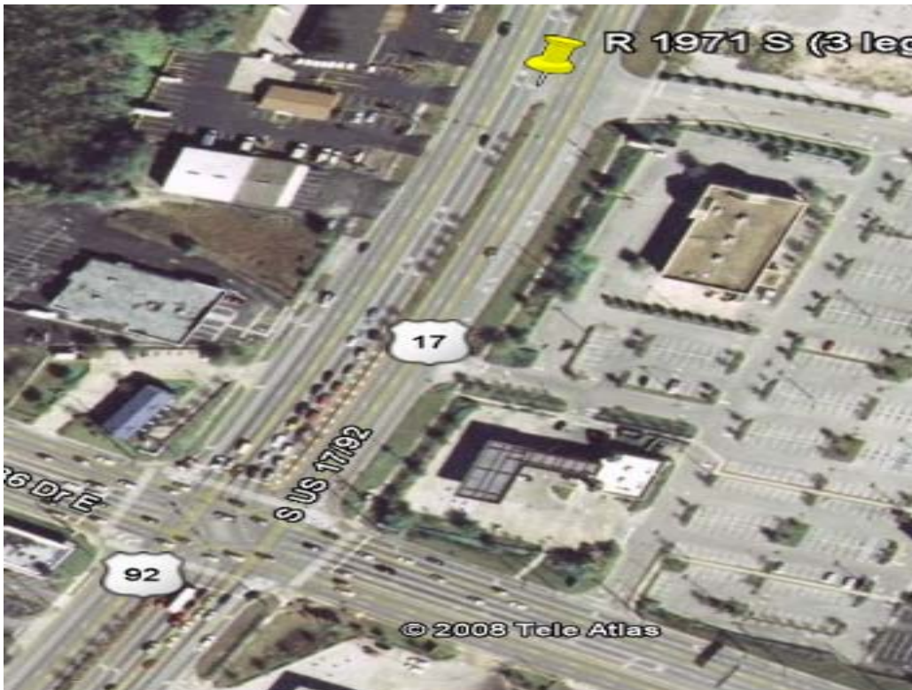
Figure 3-29: A Further View of the Unsignalized Intersection in Figure 3-28 for Better Clarification of the Extension of the Two Left-Turn Lanes to the Signalized Intersection
