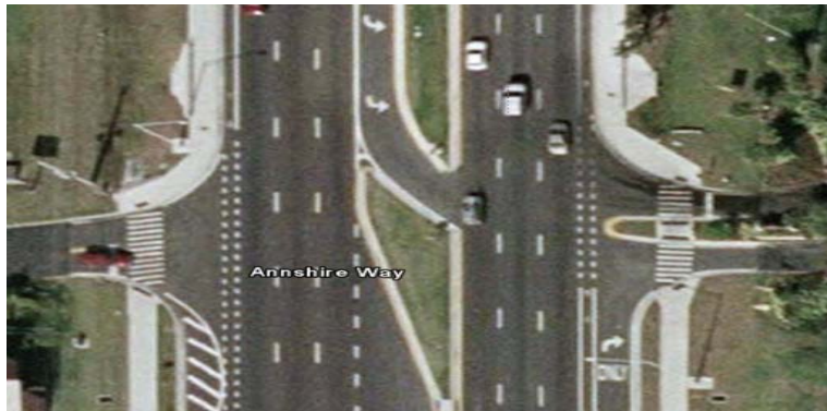
Figure 5-1: Mixed Median Type on the Major Road (Directional from One Side, and Closed from the Other Side) (Retrieved January 20, 2008, from Google Earth)
