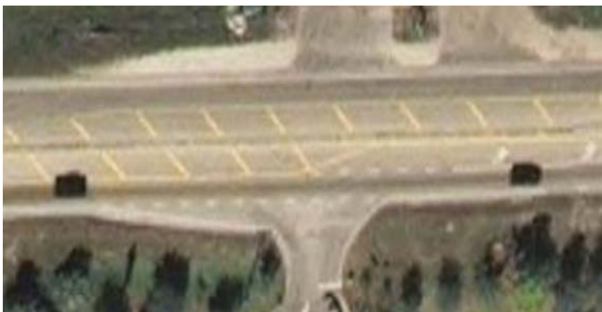
Figure 3-12: A 2x2 Four-Legged Unsignalized Intersection with Pavement Markings as a Median
