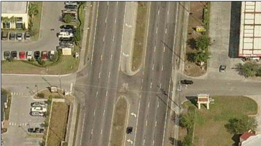
Figure 3-6: A 2x6 Four-Legged Unsignalized Intersection with an Open Median
