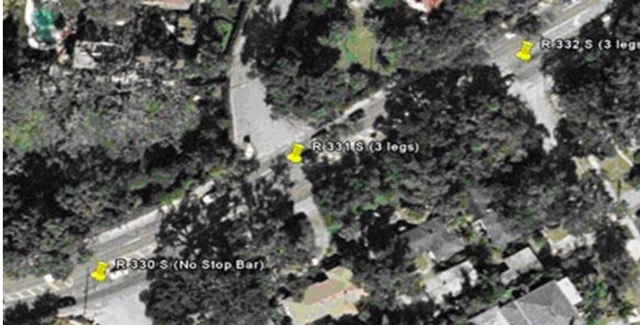
Figure 3-15: Aerial Image from “Google Earth” for 3 Unsignalized Intersections in Orange County where Difficulty was Encountered in Identifying their Geometry due to Tree Blockage
