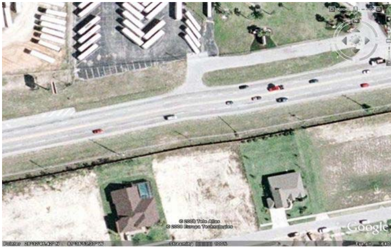
Figure 3-9: A 2x4 Three-Legged Unsignalized Intersection with an Undivided Median
