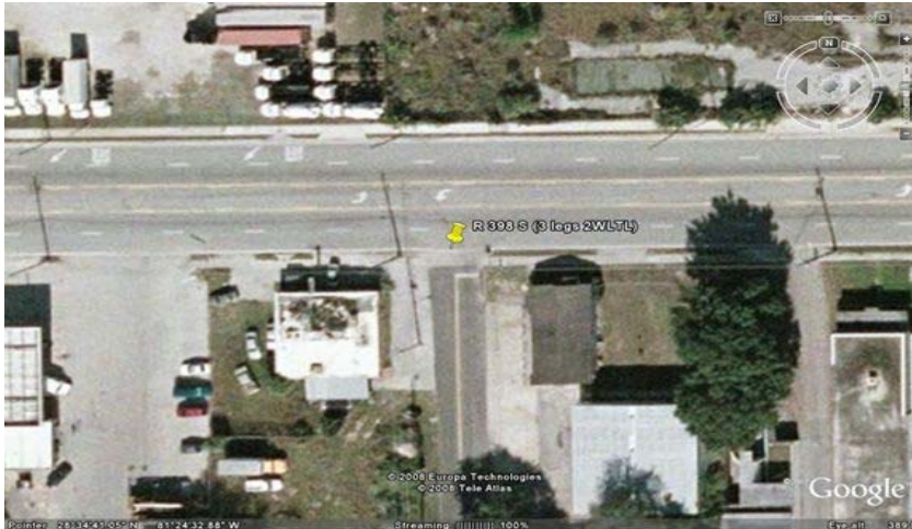
Figure 3-7: A 2x4 Three-Legged Unsignalized Intersection with a Two-Way Left Turn Lane Median
