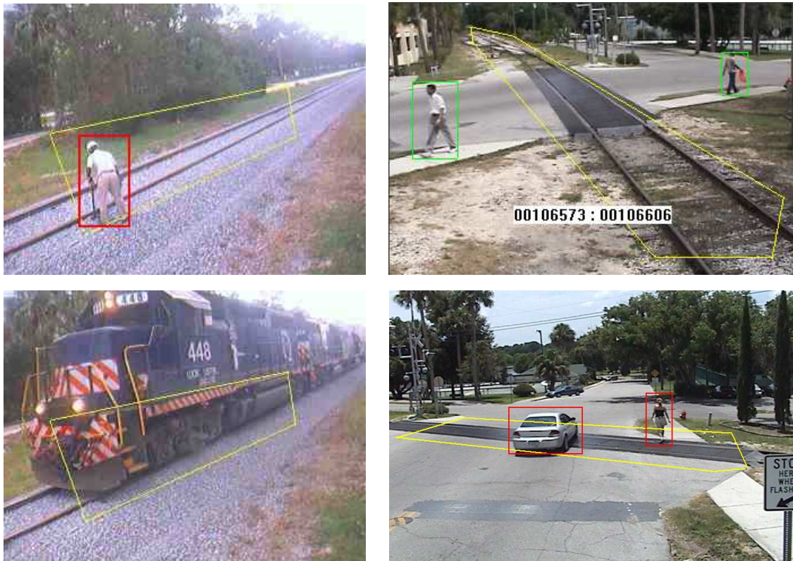
Figure 6.1: KNIGHT at Railroads: A danger zone is defined through a Graphical User Interface (GUI) and objects are warned as they enter the danger zone. The bounding box of people and vehicles, (but not of trains) turn red as they enter the polygon defining the danger zone.
