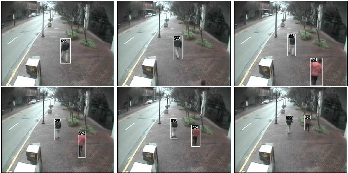
Figure 4.5: Orlando down town. Two persons being tracked on a cloudy day (low illumination).
