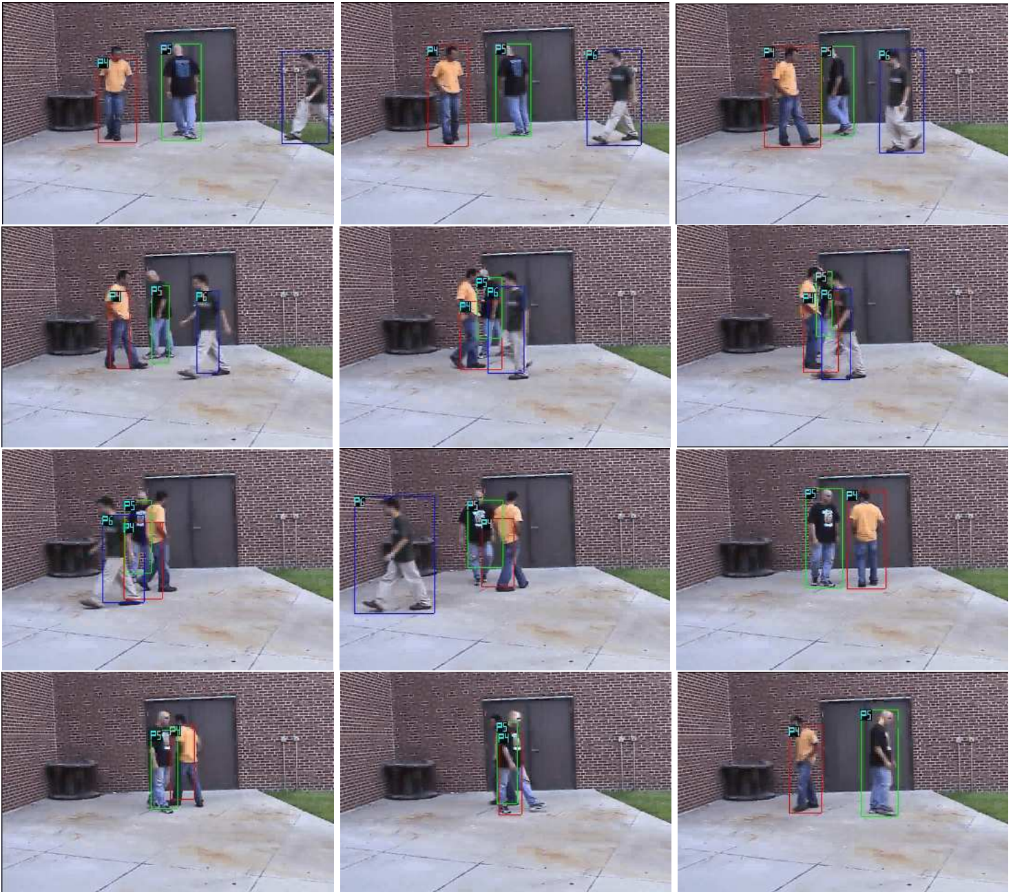
Figure 4.4: Tracking results in a single camera. The tracker is capable of handling multiple occluded people.
