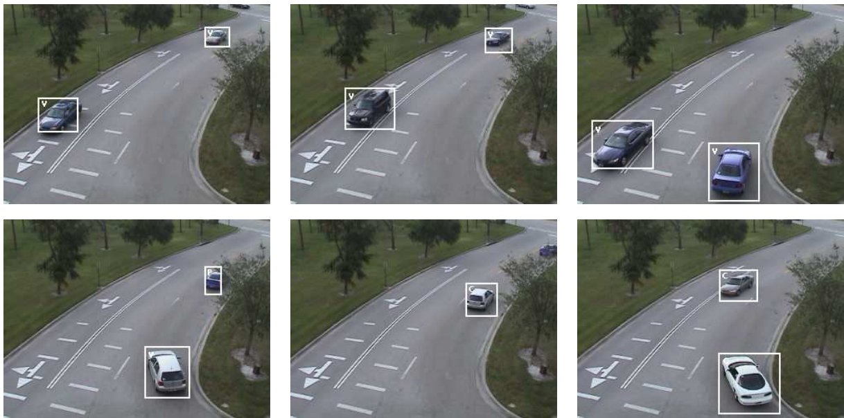
Figure 3.7: Moving object classification results from sequence 3. Note that in row 2, first image the car has been misclassified due to occlusion from the tree branches.
