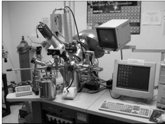
Figure 4.15 Physical Electronics 5400 ESCA XPS
