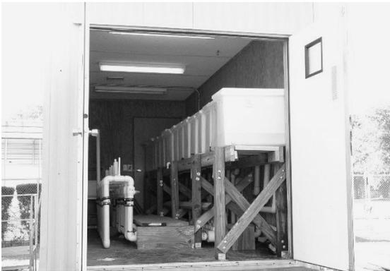
Figure 8.4 Electrochemical noise trailer
