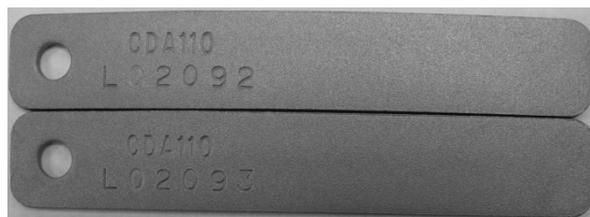
Figure 8.7 Photographs of typical copper coupons before exposure to inhibitors
