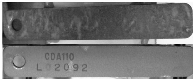
Figure 8.9 Visual comparison of surface scales on Phase III copper coupons
