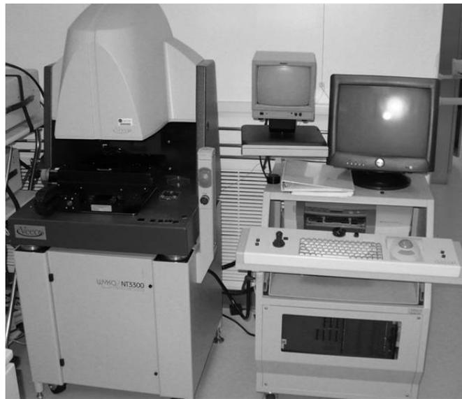
Figure 4.13 WYKO NT 3300 optical profiler
