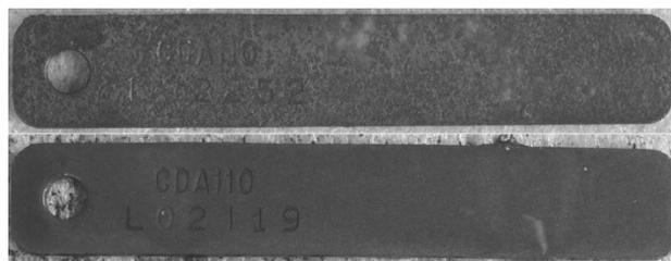
Figure 8.10 Visual comparison of surface scales on Phase IV copper coupons
