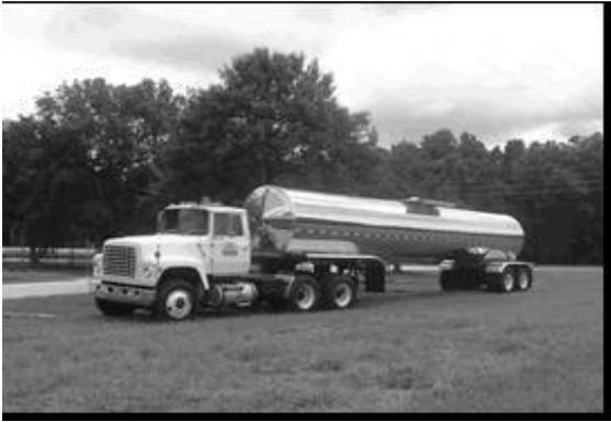
Figure 4.1 Truck and stainless steel trailer used to haul raw surface water
