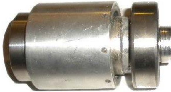
Figure 12: Completely Assembled Magnetic Bearing in Shifted Position
