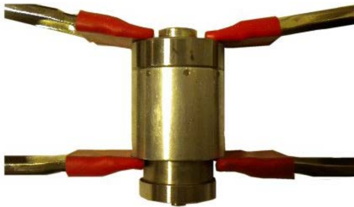
Figure 13: Completely Assembled Magnetic Bearing Forced into Alignment
