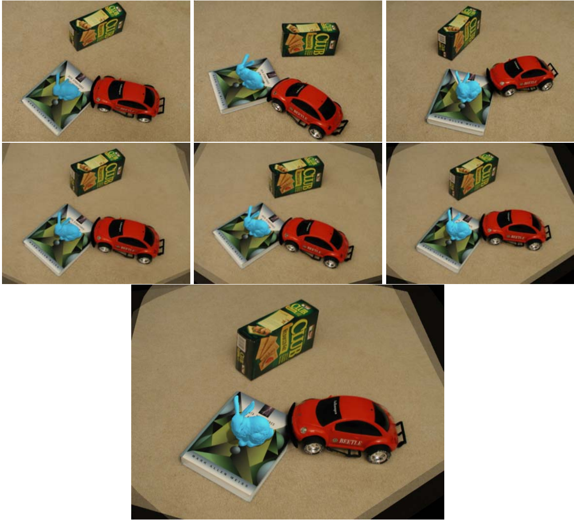
Figure 6.8: Augmenting 3D objects in tri-view morphing. Top: three original images with the augmented object (“Bunny” model from Stanford University). The 3D model is accurately augmented on the top of the book. Middle: a series of synthesized virtual views with the augmented object can maintain geometric correctness in the morphing procedure. We also generate the shadow of model and cast it on the book by assuming a light source. The bottom image is an enlarged result.
