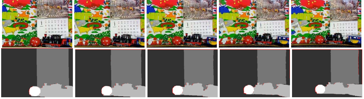
Figure 4.20: The segmentation results for the mobile-calendar sequence. The red pixels are occluded pixels.
