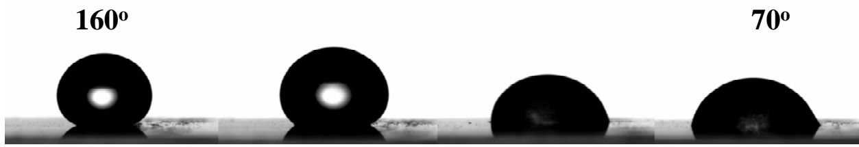
Figure 2.8 The change of water contact angle Vs temperature on a hydrophobic/hydrophilic switchable surface.
