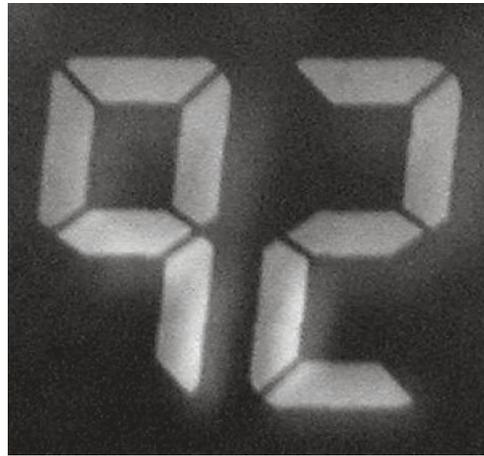
Figure 25: The displayed image using a dye-doped T-PDLC reflective display. Black dye concentration: 2%, LC/polymer mixture: NOA65:E48=40:60,  $d=6.7 \mu\text{m}$ , and  $V=20 V_{\text{rms}}$ . A white paper was placed behind the bottom substrate to act as a diffusive reflector.
