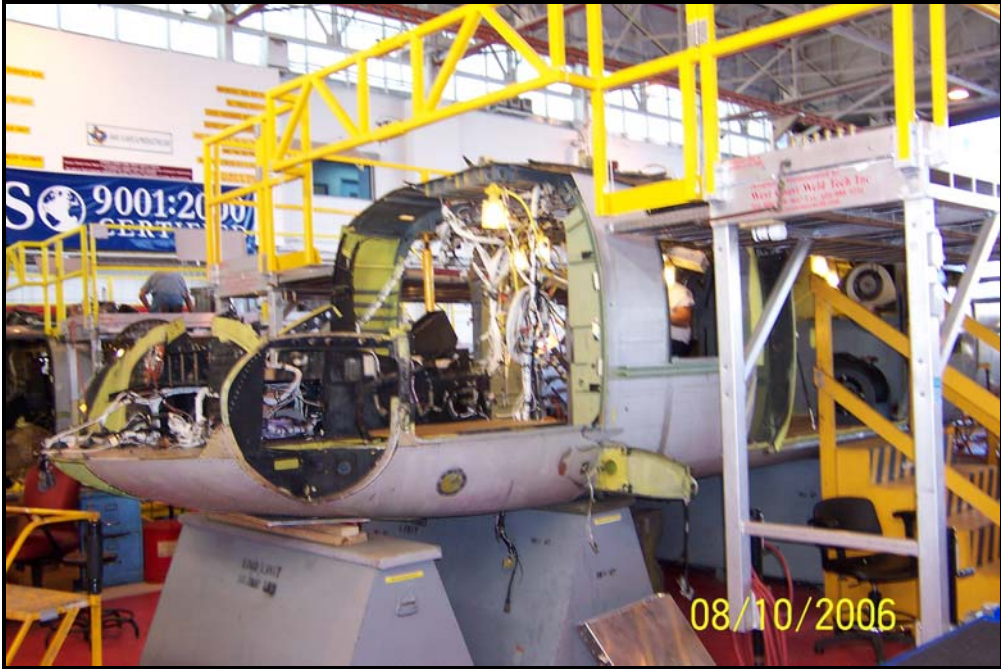
Figure 2: Forward View of Electrical Upgrades to UH-60A
