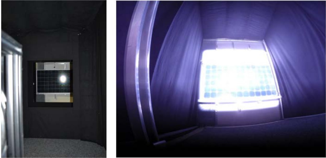
Figure 61. Sinton FMT-350 solar simulator; (left) view from the light source toward the module and (right) module during illumination.
