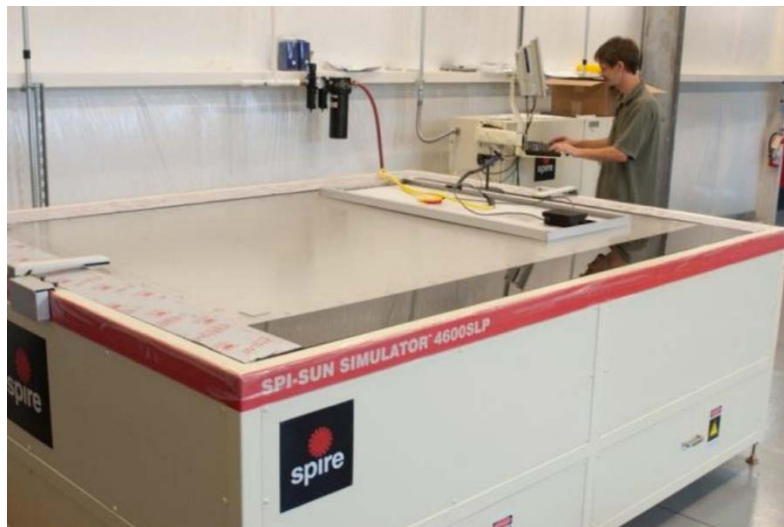
Figure 62. Spire 4600 solar simulator. Modules are placed face down on the glass.
