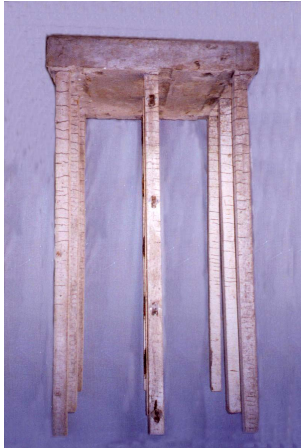
(a) Cracking on the pile foundation
