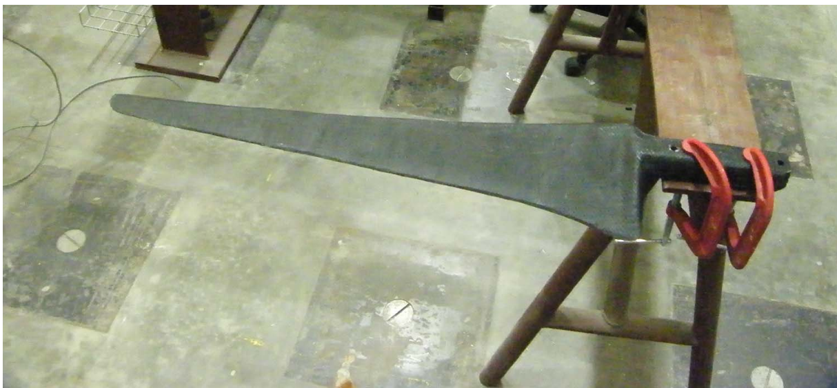
Figure 5.4: Photograph of the wind turbine basalt fiber blade.
