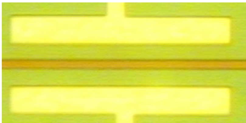
Figure 3.10: Optical microscopy image of CNT electrode fabrication steps (after EBL and develop). This figure shows a straight window is opened by EBL.
