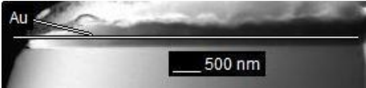
Figure 23: HAADF-STEM micrograph of wedge shaped Au. From left to right, the thickness increases. The corresponding intensity profile (line scan) is shown in Figure 24. The layer above Au is Pt from the FIB deposition process, and the substrate below is \text{LiTaO}_3 .
