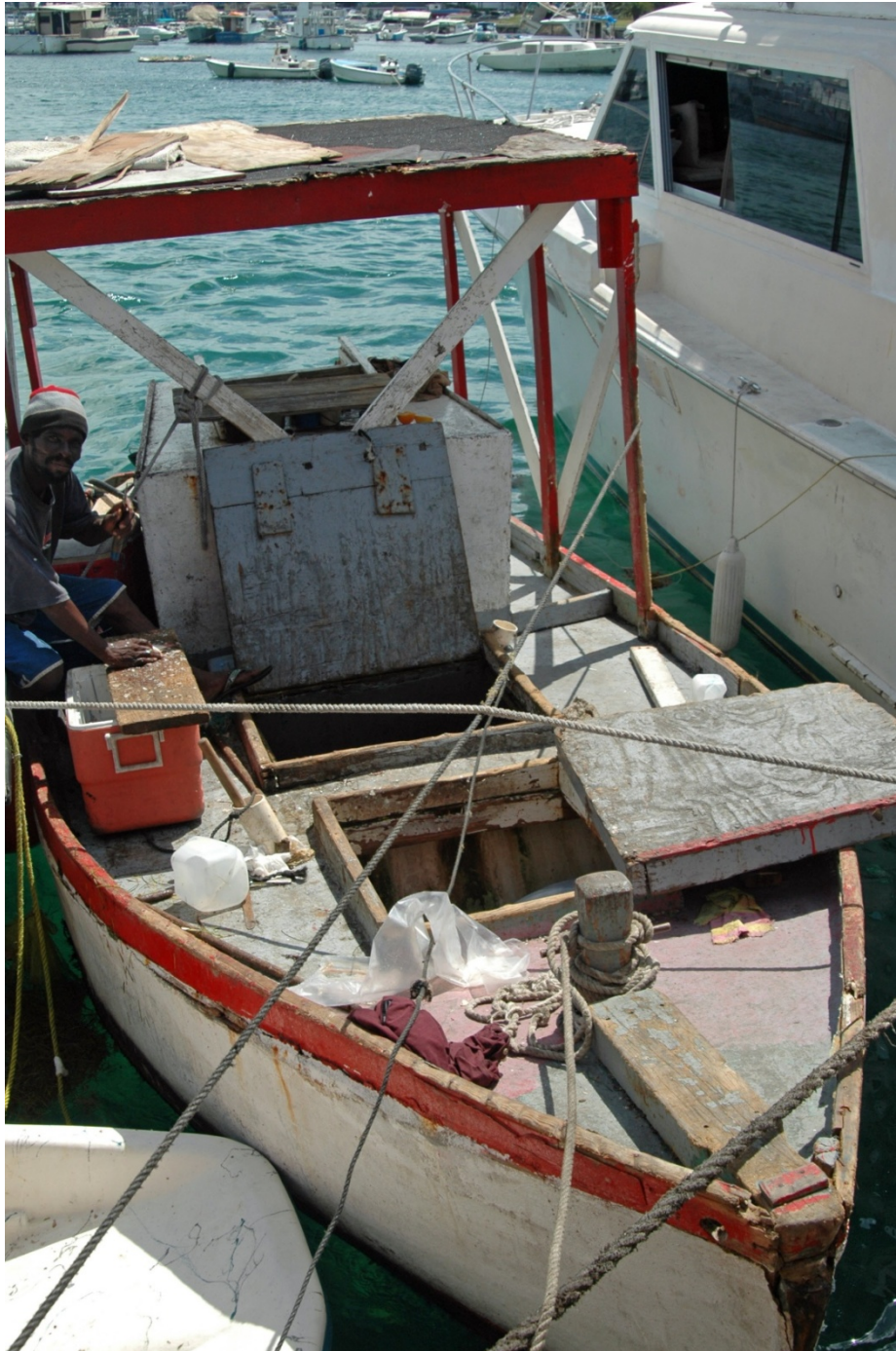
Figure 9: The Lively Hope . Bahamian fishing vessel with non aerated live well. Photo courtesy of David Smith.
