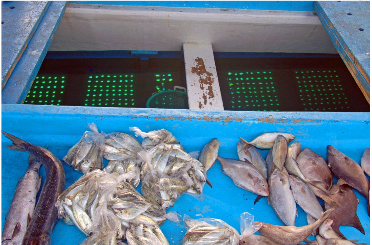
Figure 12: Close up of live well on “ The Surprise ”. Note the holes in the bottom of the well to allow for water exchange. Photo courtesy of David Smith.
